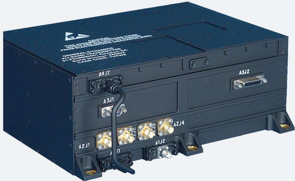
General Dynamics' HRT150 Ku-Band Transmitter provides a solution for delivering large amounts of data from a spacecraft in one small package. Standard operation is Tracking and Data Relay Satellite System (TDRSS) Ku-Band, with options available for X-Band and Ka-Band. The transmitter is compatible with NASA's TDRSS KuSAR high-rate return link receiving systems.
