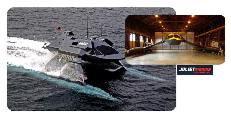
Small Waterplane Area Twin Hull (SWATH) provides excellent sea keeping through Sea State 4, allowing operation of larger payloads not normally available on small surface vessels
