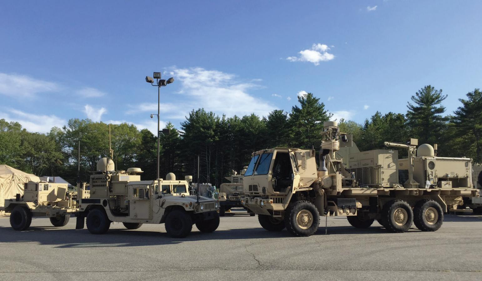
A TCN-L (on left) represents a significant step forward in creating a more agile WIN-T network at reduced cost as compared to the initial TCN (on right). Integrated onto a HMMWV, a TCN-L provides complete TCN capability in a greatly reduced footprint and improved transportability for expeditionary operations (C-130 roll-on/roll-off and CH-47 sling loadable) while also reducing the complexity to install, operate and maintain the system. (Photo credit: General Dynamics)
