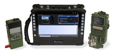
The CTS-6025 CSAR Radio Test Set is developed exclusively for use with Hook Series Radios from General Dynamics
