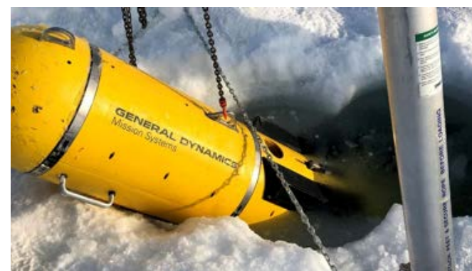
At ICEX 2020, MIT partnered with General Dynamics to demonstrate new navigation technologies by deploying the Bluefin-21 Macrura UUV under a six-foot-thick sheet of ice. (Image Credit: Dan McDonald, General Dynamics Mission Systems)
