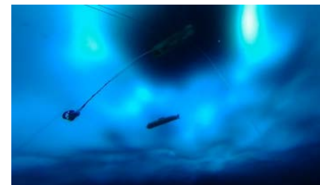
At ICEX 2020, MIT partnered with General Dynamics to demonstrate new navigation technologies by deploying the Bluefin-21 Macrura UUV under a six-foot-thick sheet of ice. (Image Credit: Dan McDonald, General Dynamics Mission Systems)
