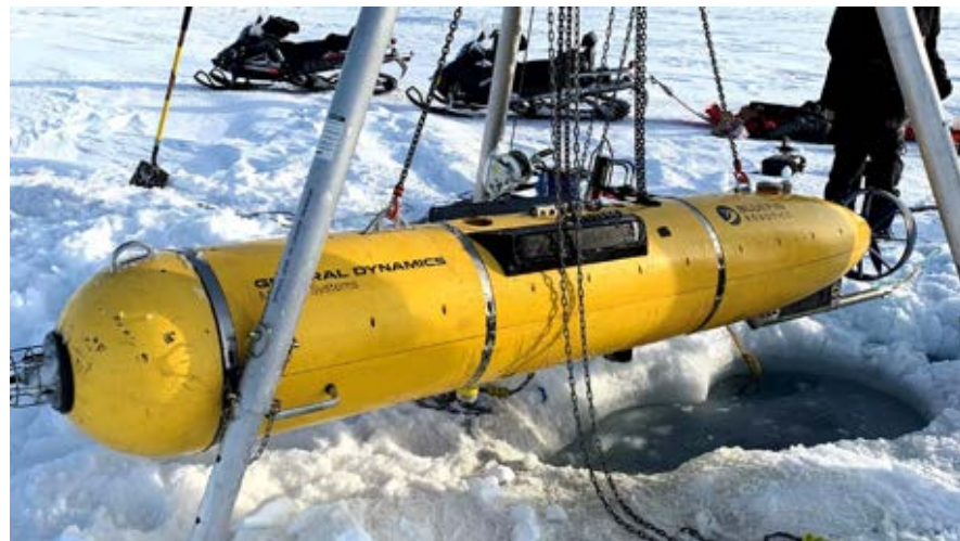
Under the ice and on top of the world. During the U.S. Navy's ICEX 2020 Exercise, one of our Bluefin-21 autonomous Unmanned Underwater Vehicles (UUVs) was put to the test in the harsh conditions of the Arctic Circle. (Image Credit: Dan McDonald, General Dynamics Mission Systems)
