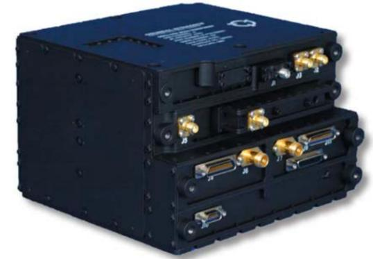
The rover also carries our [X-band solid-state power amplifier](#) (below). This highly reliable power amplifier, synchronous rectifier and power converter unit has supported all previous rover missions to the Red Planet and several other deep space destinations.
