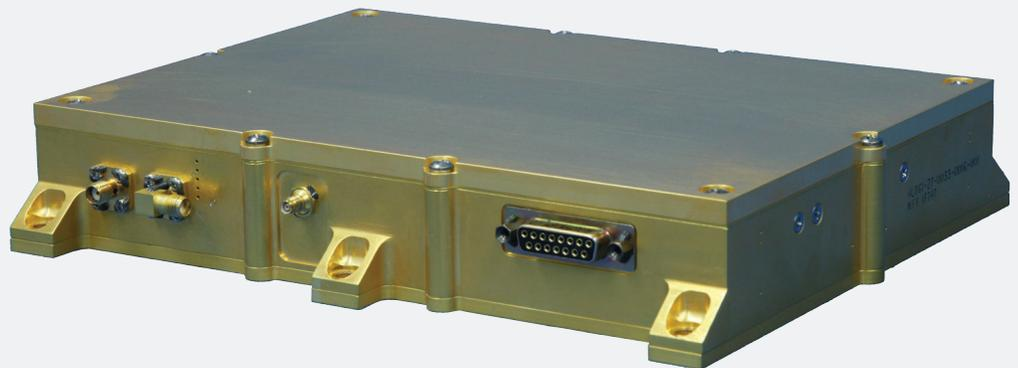
General Dynamics' space-qualified, S-Band Solid State Power Amplifier (SSPA) offers highly efficient and reliable power amplification and features an internal DC-DC power converter and voltage regulator. Operating over the 2.2 to 2.3 GHz frequency range, the SSPA serves as a companion unit to General Dynamics' Multi-Mode Standard Transponder (MST) or operates as a stand-alone power amplifier.
