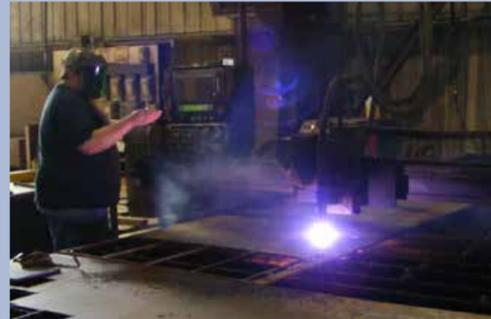
*Computer-controlled plasma cutters transform steel plate into complex shapes.*
