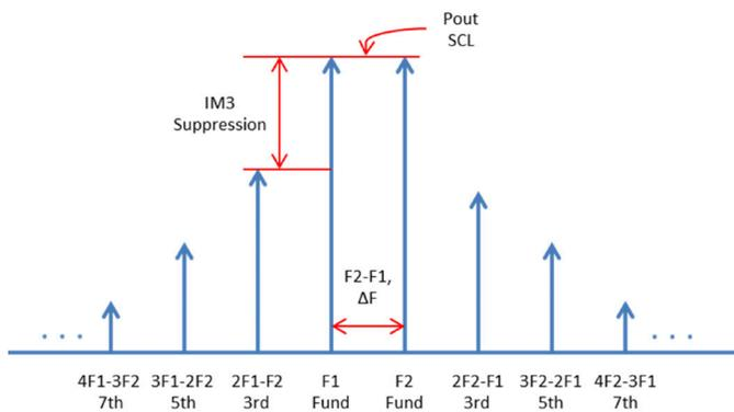
Figure 2: 2-Tone Intermodulation Spectrum
