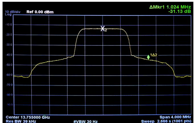
Figure 3: Spectrum Analyzer Response for QPSK Spectral Regrowth Measurement. Delta marker is positioned at 1.0xSymbol Rate
