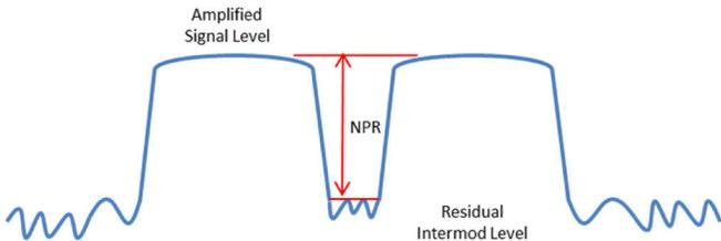
Figure 4: Typical NPR Measurement Output Spectrum
