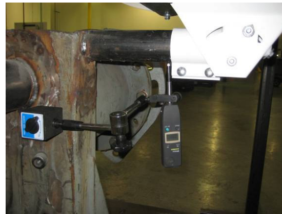
Image A.4 Mast Pipe Indicator
