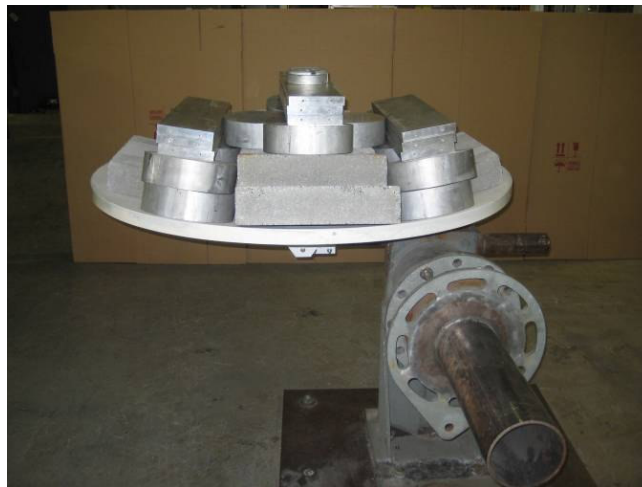
Figure 4.5.1 Survival Wind Load
