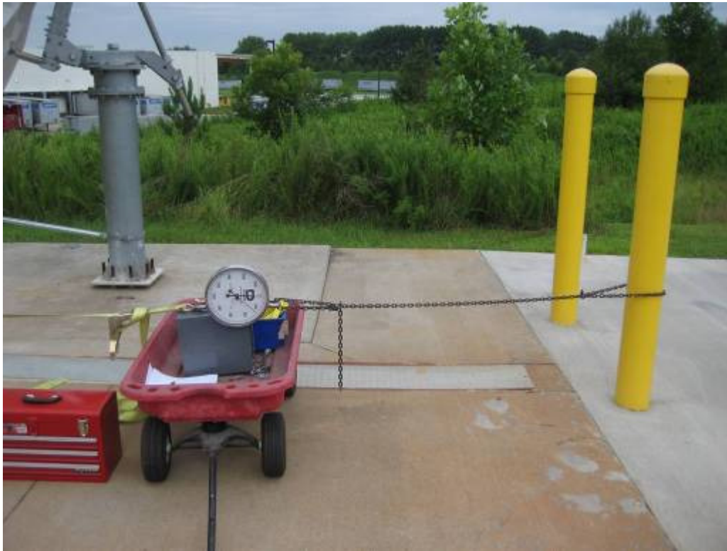
Figure 14: Mast Pipe Deflection Test Setup 3
