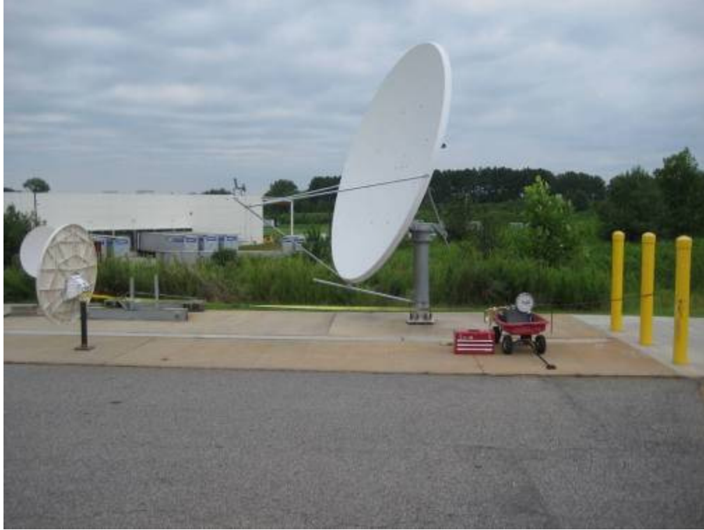
Figure 12: Mast Pipe Deflection Test Setup 1
