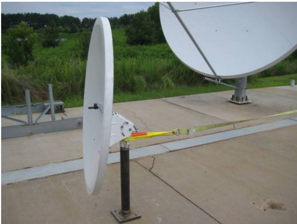
Figure 13: Mast Pipe Deflection Test Setup 2
