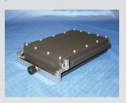
The  $\mu$ RMS-SS is a removable solid-state cartridge designed for harsh environments. The  $\mu$ RMS-SS provides up to 256 gigabytes of non-volatile storage allowing users to tailor  $\mu$ RMS-SS capacity to their affordability requirements.
