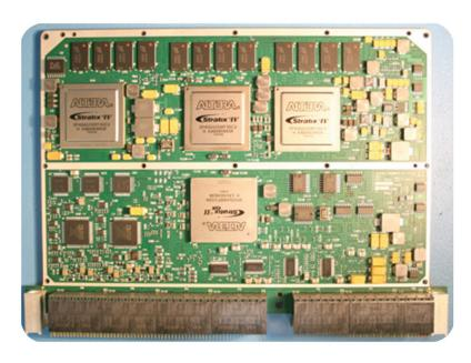
Available with up to four FPGA devices to support a wide array of sensor and video processing applications
