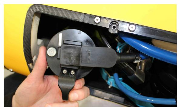
The Bluefin-9's Removable Data Storage Module (RDSM) is a field-swappable module that processes and stores data collected by integrated sonar, camera and environmental sensors. An operator is able to recover and redeploy their vehicle in 30 minutes or less and have reviewable or actionable data in-hand immediately.
