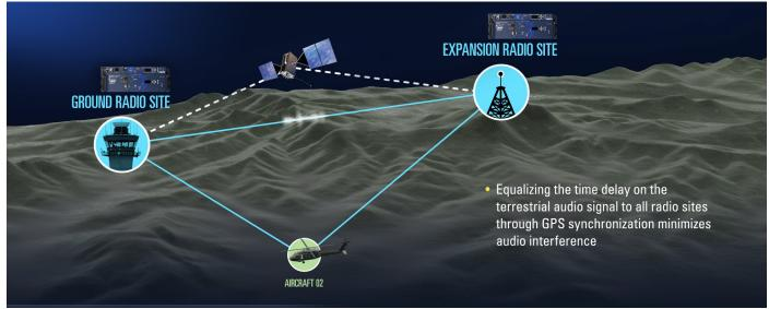
Challenge: Terrestrial Audio delay between multiple transmitter sites introduces an echo in the pilots headset.
