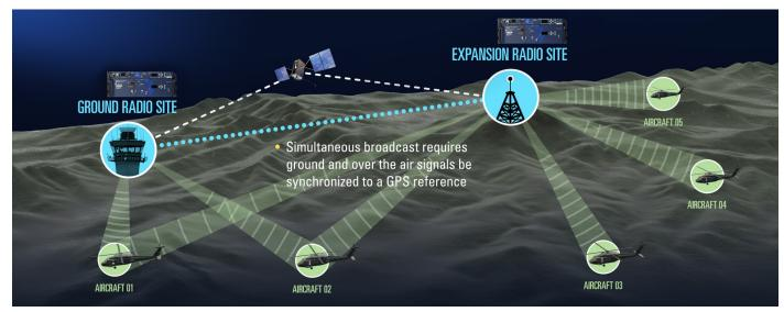
**Challenge:** Simultaneous broadcast from multiple transmitters can generate audio distortion in the cockpit if the transmitter frequencies are not synchronized.
