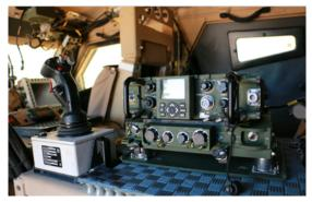
AN/PRC-155 Manpack Radio – Single Vehicle Mount
