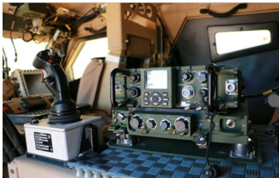
AN/PRC-155 Manpack Radio – Single Vehicle Mount
