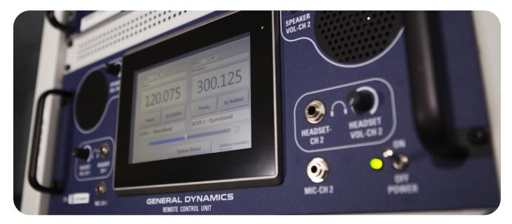
Remotely control up to two remote CM-300/350 (V2) transceivers over a network connection
