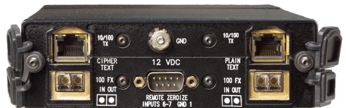
The back panel of the TACLANE-Nano Adapter Module mirrors the back panel of the TACLANE-Micro (KG-175D) for easy crypto replacement
