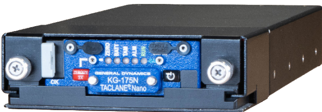
TACLANE-Nano (KG-175N) Adapter Module (for KG-175D)
