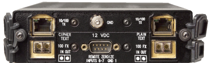
TACLANE-Micro (KG-175D) Back Panel
