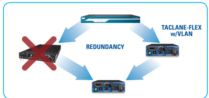
Redundancy provides failover capability. When a path through an INE is no longer available, traffic is re-routed to the next best route.
