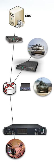
The GDS enables HAIPE devices to locate other registered HAIPE devices on the network, automating configuration and providing redundant routes.
