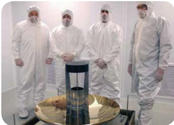
General Dynamics has proven capability to design, manufacture, polish and integrate optical components and assemblies up to 1.5 meters in diameter.
