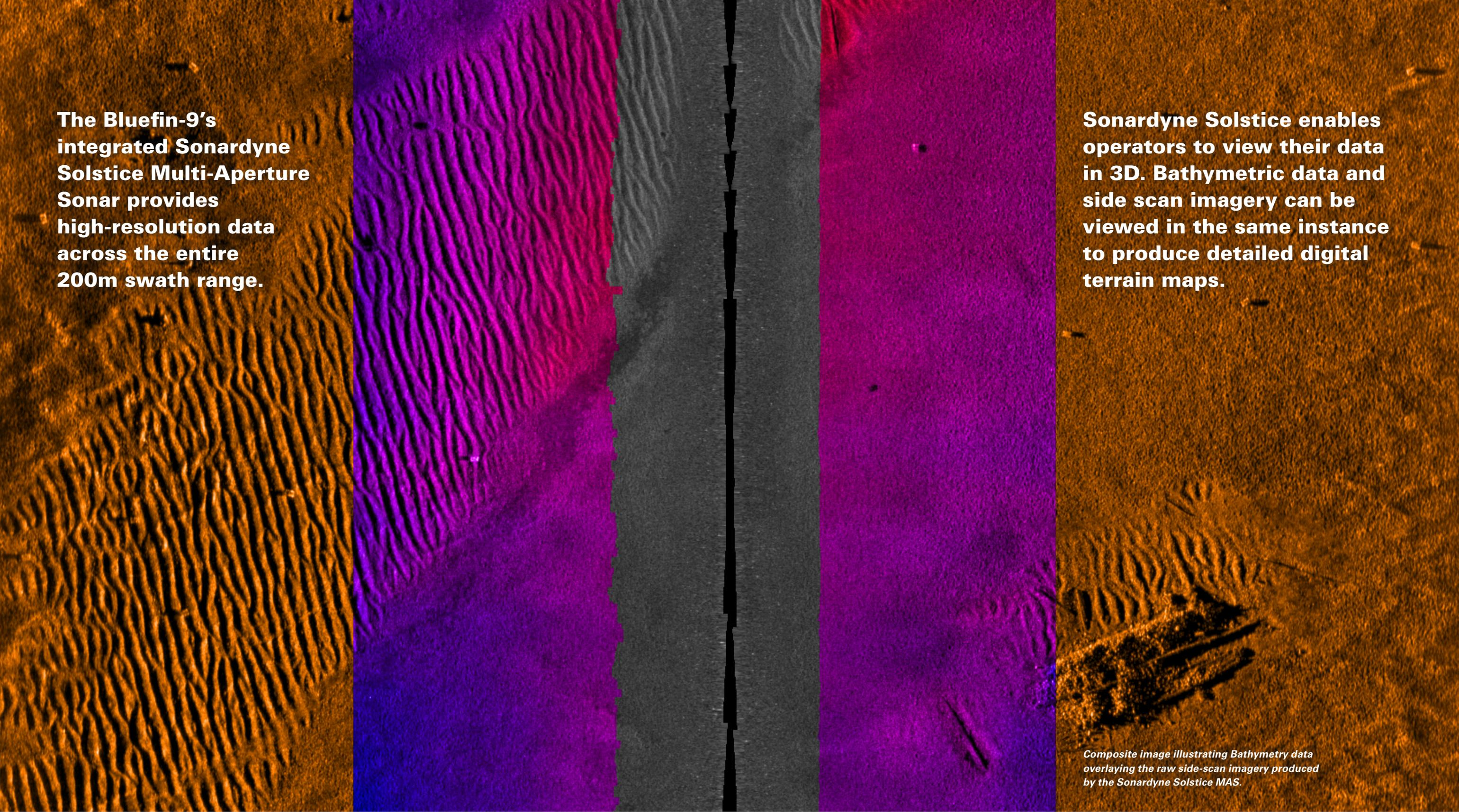
**The Bluefin-9's integrated Sonardyne Solstice Multi-Aperture Sonar provides high-resolution data across the entire 200m swath range.**
