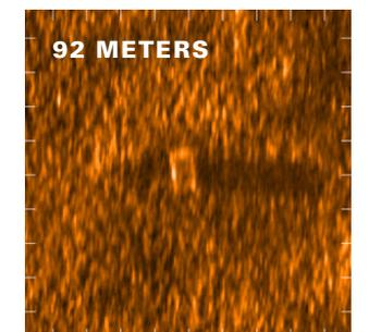
High-resolution and positive feature identification across the full swath range. Images here show lobster pots at 22, 47, 72 and 92 meters from the Bluefin-9 UUV.
